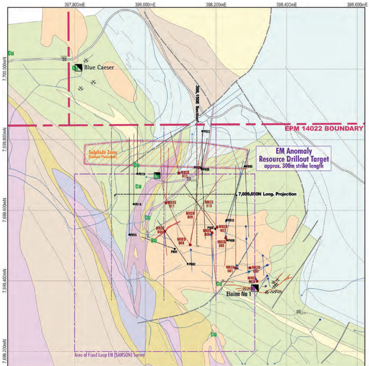
Figure 5: Drillhole location plan – the Elaine prospect, Mary Kathleen JV Project with Goldsearch Limited. Note the area of the EM anomaly suggesting a target area for resource drillout of at least 300m strike length.
