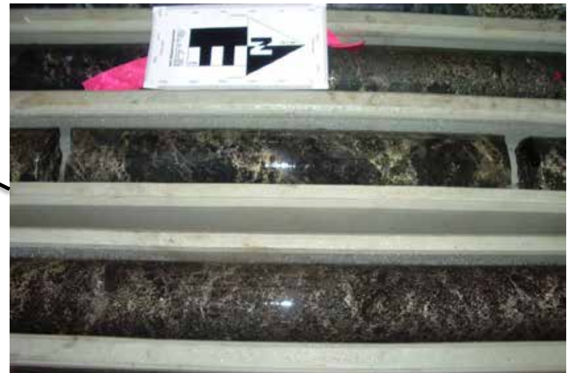
MKED036 – ~240m - Elaine copper-gold resource – pervasive sulphide mineralisation, sulphide breccia - dominated pyrrhotite + chalcopyrite +/- pyrite – co-incident with resistivity low EH4 anomaly.
