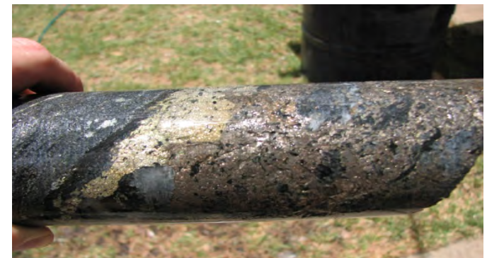
2012 – Diamond drilling – chalcopryite sulphide mineralisation intersected in core
