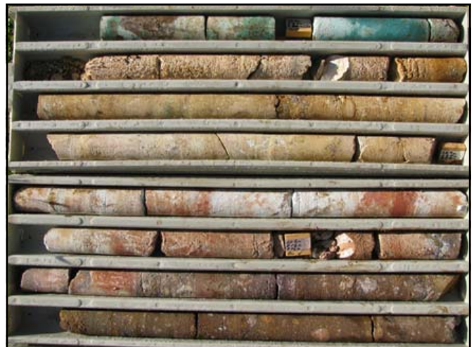
Figure 4. MDD006 core recovered in the target breccia from 50 metres and continues at depth to 78 metres. Yellow brown rock in bottom metres is supergene chalcocite (copper sulphide) breccia from 60.5 metres and confirms the extension at depth of the Mt Dorothy sulphide breccia. The top metre is green pseudomalachite in breccia. The brown metres at the bottom of the tray average 10.5 % copper.
