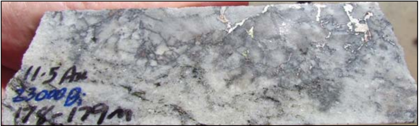
An example of the high grade gold bismuth mineralisation in the core of the Elaine copper cobalt REE Thorium deposit. Intercept is 11.5g/t gold, 2.3% bismuth, 0.28% copper from 178 to 179 metres.
