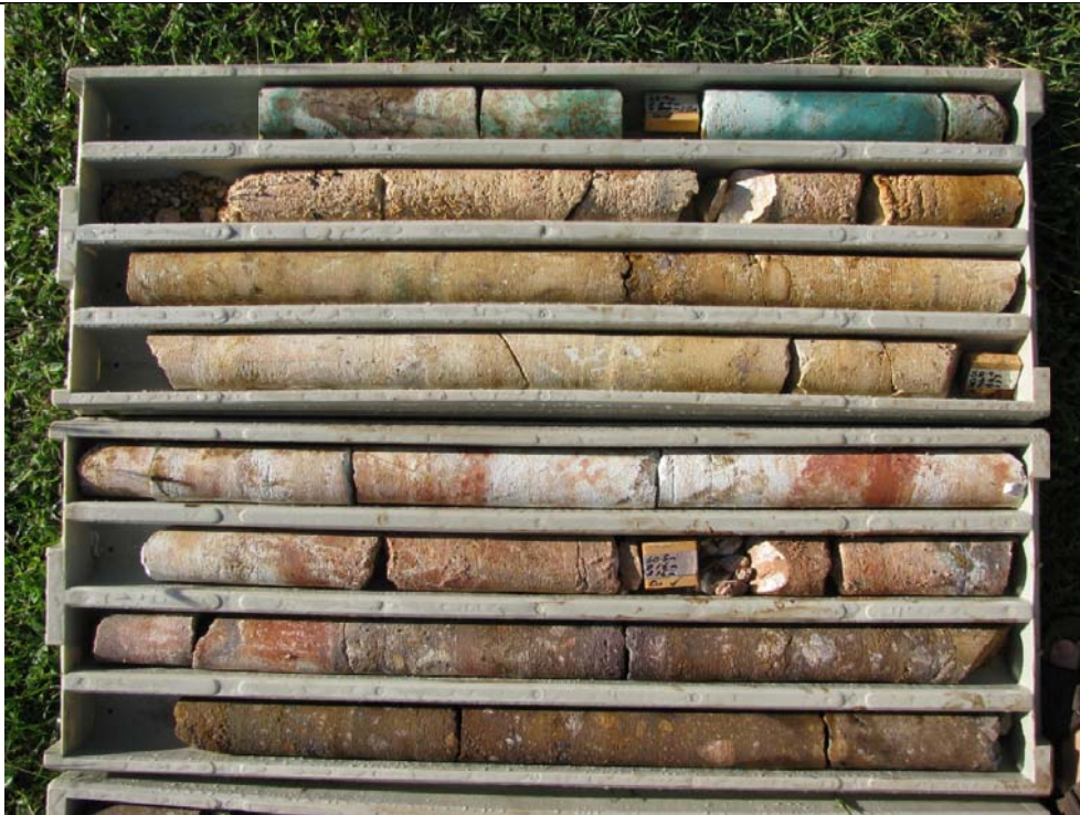
Figure 1. MDD006 – Core recovered in the target breccia from 50 metres and continues at depth to 78 metres. Yellow brown rock in bottom metres is supergene Chalcocite (Copper Sulphide) breccia from 60.5 metres confirms the extension at depth of the Mt Dorothy sulphide breccia. The top metre is green pseudomalachite in breccia. The brown metres at the bottom of the tray average 10.5 % copper.
