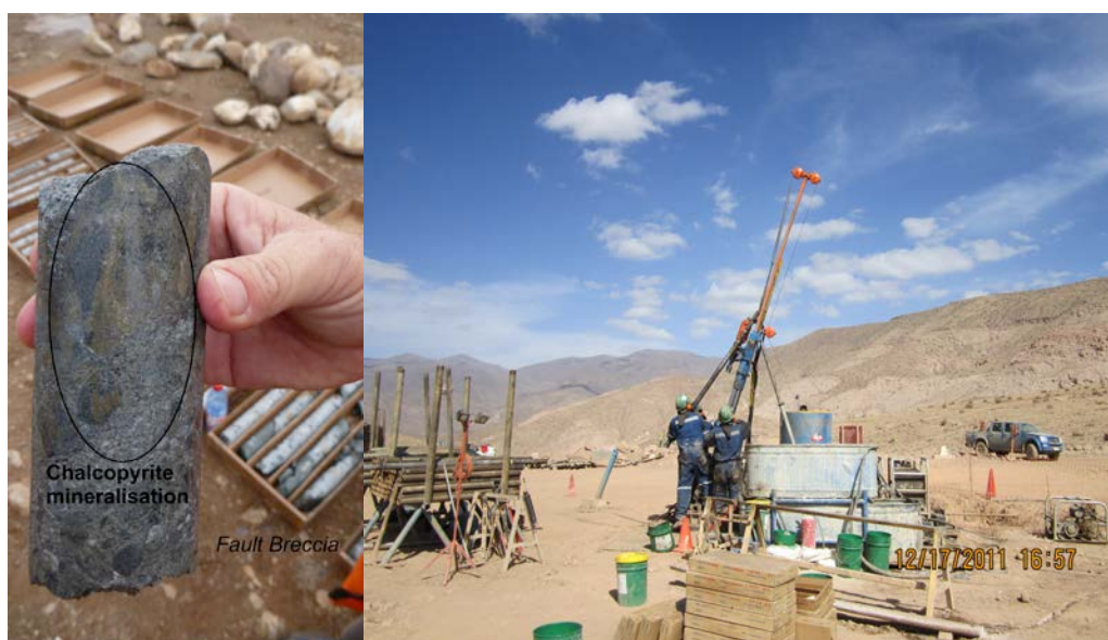
Copper Mineralisation from CAND0005 and Energold drillrig set up.
