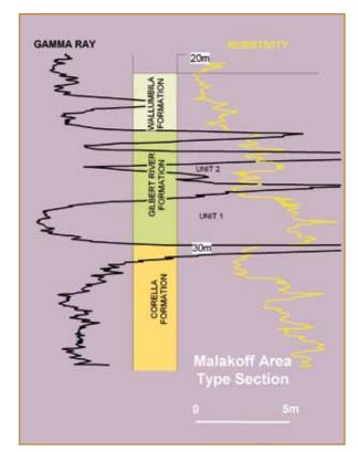
Figure 9: Malakoff Area Typical Drill Section
