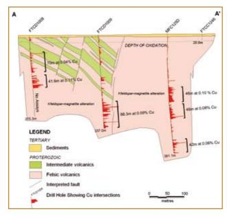
Figure 6: FC4 Prospect Simplified Cross Section
