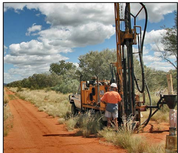
Vehicle-mounted light aircore drilling rig used for alluvium sampling at Charley Creek
