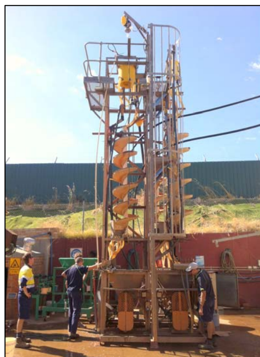
Spirals used for wet plant pilot testwork at Allied Mineral Laboratories in Perth, WA
