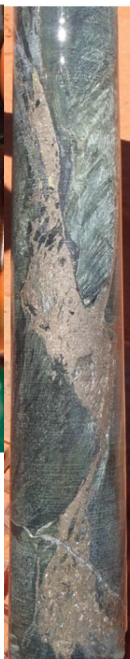
Figure 13b MTD011. Clasts of massive nickel sulphide (with copper sulphide) in breccia zone in dunite. The clast may be remobilised from a nearby body of massive sulphide.
