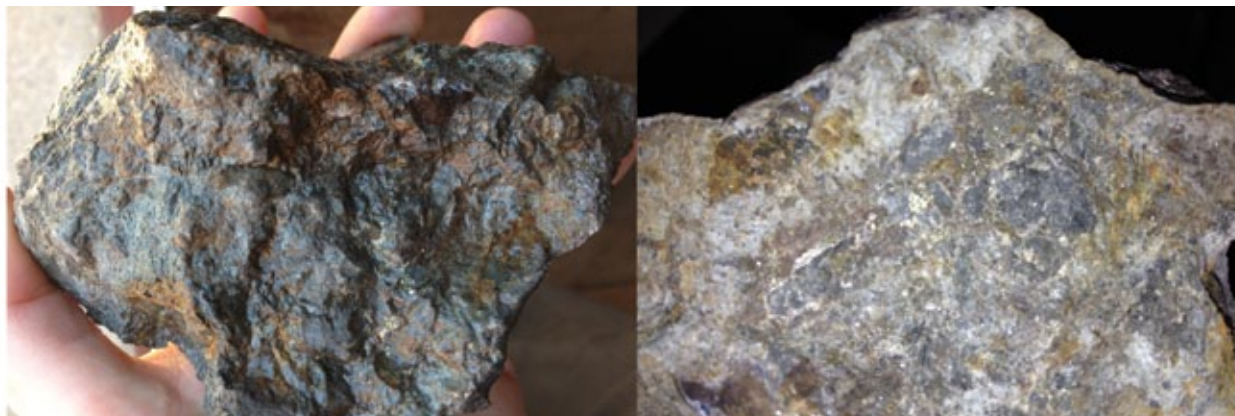
Figure 4. Examples of mineralised rocks from the Coronation area. Malachite (green colour) stained weathered breccia (left) and silica altered pyrite-chalcopyrite-bearing rock (right).
