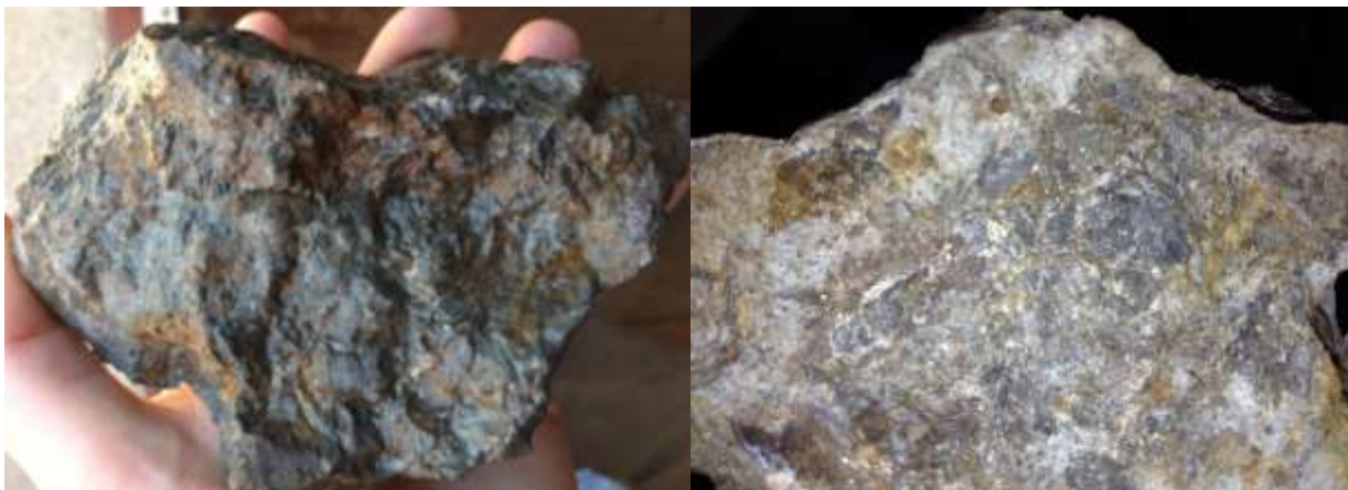
Figure 3. Examples of mineralised rocks from the Coronation area. Malachite (green colour) stained weathered breccia (left) and silica altered pyrite-chalcopyrite-bearing rock (right).
