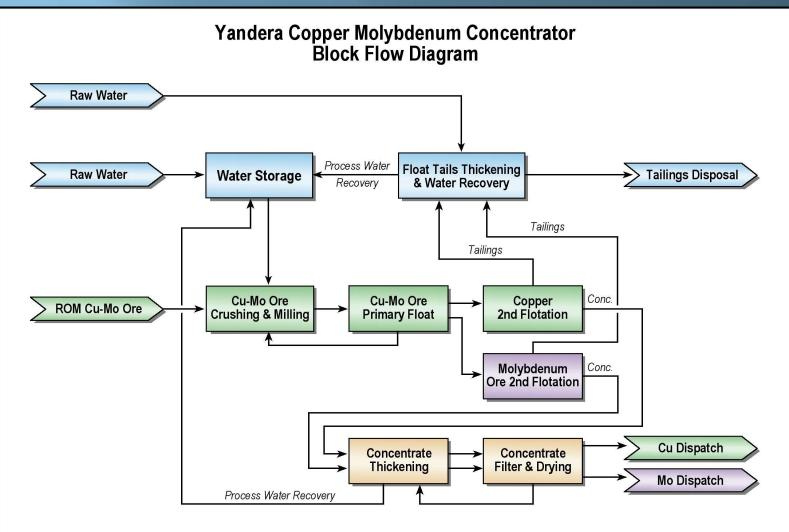
Production of separate copper and molybdenum concentrates
