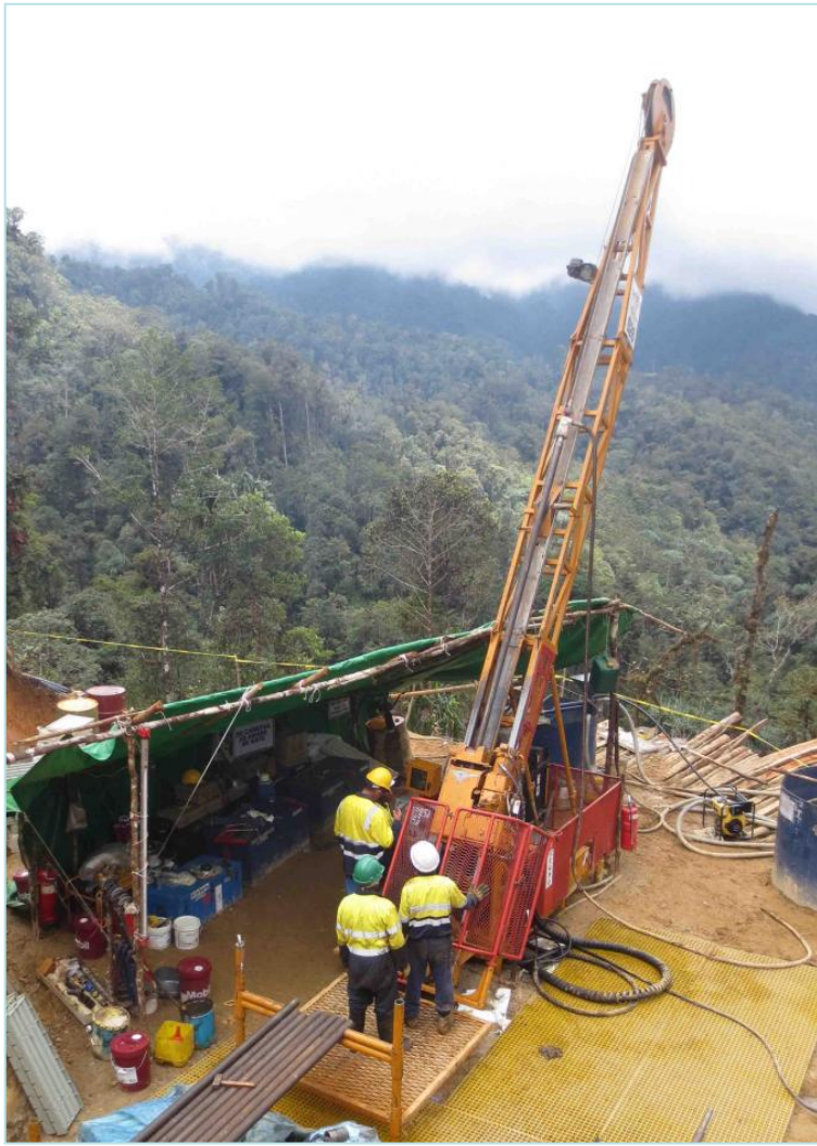
Rig drilling YD 551 on azimuth of 150° (AMG), depressed at -60°
