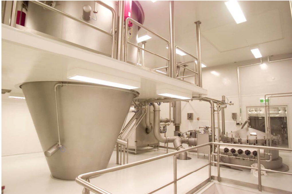
Central sections of spray drier
