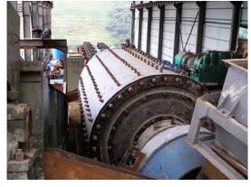
Figure 5 : Ball Grinder and Flotation Mill at Damajianshan Mine Beneficiation Plant
