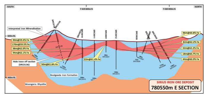
Figure 4. Cross Section through Sirius Deposit at 780550m E
