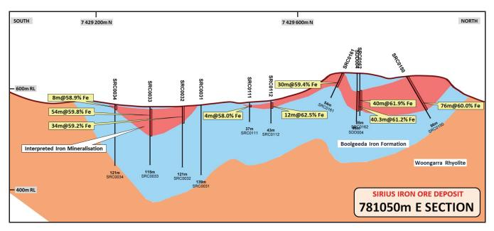
Figure 5. Cross Section through Sirius Deposit at 781050m E
