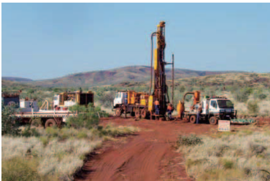
Fig 3 RC drilling at Marillana
