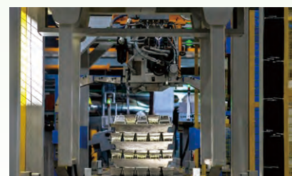
Automated transportation of tin ingots in Yunnan green smelting factory.
