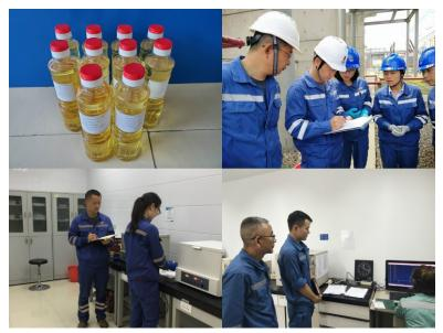
The assessment activity composed of anonymity test, on-site sampling transformer oil and on-site chromatographic analysis and operation for transformer oil, covering sampling, testing, analysis and other procedures of the electric power oil inspection. The activity focused on the understanding of the technical standards by professionals in various segments, as well as the standardization of testing and operation, and accuracy of test results, etc.
