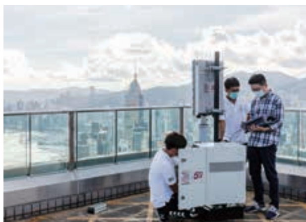
3 Hong Kong engineers testing a 5G radio base station on a rooftop
