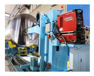
Anti-wave Plate TIG Automatic Welding Robot Workstation
