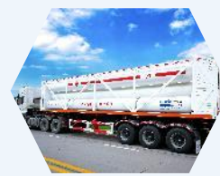
▲ Hydrogen Tube bundle trailer ▲ Hydrogen storage tank
