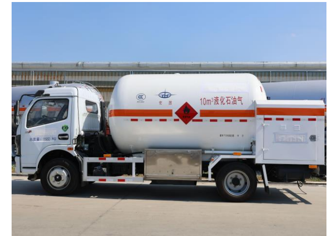
LPG Pump Tanker for Micro-pipe Network
