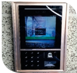
Intercom access control with camera
