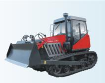
The walking device is a crawler type, mainly used for pulling and driving various supporting equipment, agricultural machinery for completing agricultural operations, various earthwork operations, transportation operations and fixing operations.
