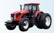
The walking device is wheeled, mainly used for pulling and driving various supporting equipment, agricultural machinery for completing agricultural operations, various earthwork operations, transportation operations and fixing operations.
