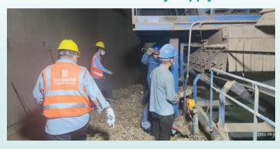
deficiencies in equipment in a timely manner. In the photo, the patrolling employees is overseeing urgent repair by maintenance workers under high temperature conditions to clear up blockage in the biomass fuel conveyor bridge identified during the inspection patrol, so as to restore normal operation of the conveyor belt as soon as possible.
