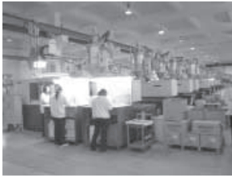
Picture 1 Resin are conformed into different required forms by an automatic moulding machine.
