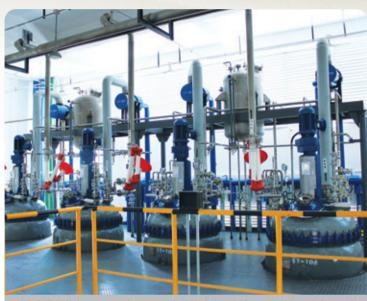
重慶康樂製藥有限公司三車間303生產線搪玻璃反應罐,用於替加環素產品生產 Chongqing Kangle Pharmaceutical Co., Ltd.\* 303 production line glass-lined reaction tank for producing tigecycline products
