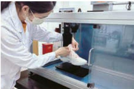
Thermal and moisture permeability test of shoes
