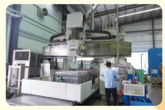
CNC machine is processing machining process on a large mould base
