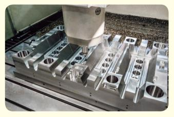
A complicated mould base is undergone machining
