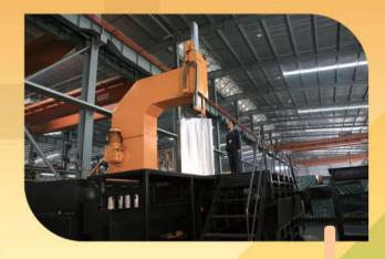
Using the vertical band saw to cut away the residual material in order to save time and cost in the milling process
