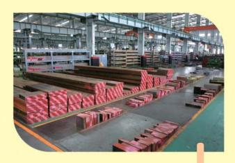
Using the colour code to distinguish different steel types systematically
