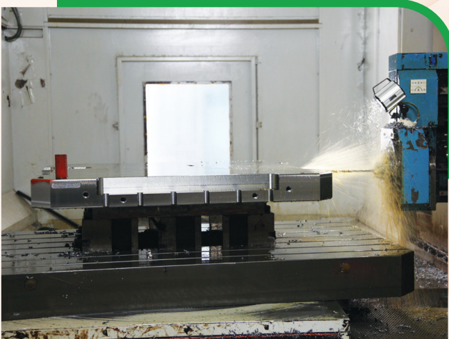
加工中心正為一件大型模架進行加工 A CNC machining centre is processing the machining for a large size mould base
