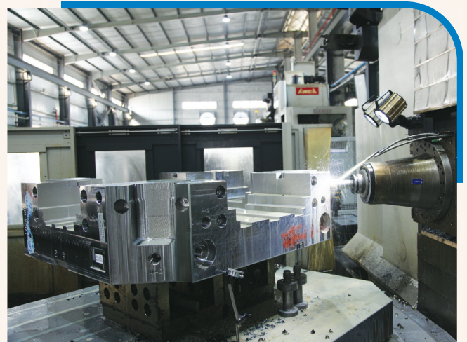
卧式加工中心正為一件大型非標模架進行 切削形框及精孔 A horizontal machining centre is processing the pocketing and precision holes for a large size custom-made mould base
