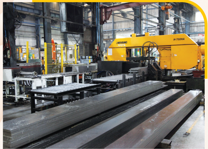
鋼材板件於加工前在切割區被切割成粗形 Steel blocks are sawed into rough shape at the cutting area before rough machining
