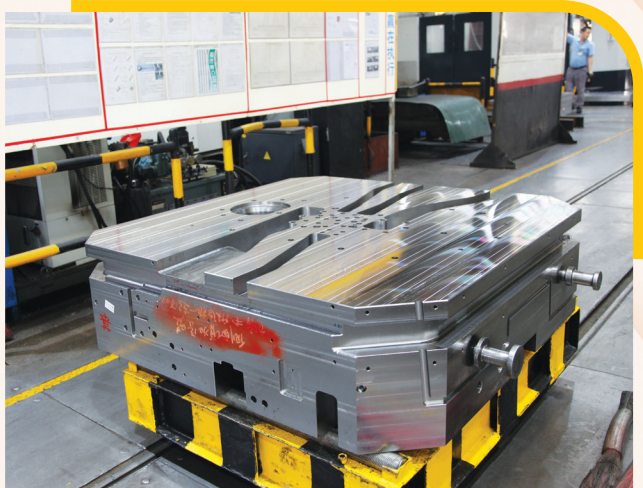
大型非標模架部分 Part of a large size custom-made mould base
