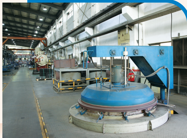
提供熱處理加工服務的回火爐 A tempering furnace for providing heat treatment service
