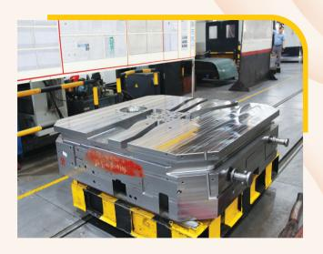
▼大型非標模架部分 Part of a large size custom-made mould base
