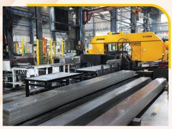
鋼材板件於加工前在切割區被切割成粗形 Steel blocks are sawed into rough shape at the cutting area before rough machining
