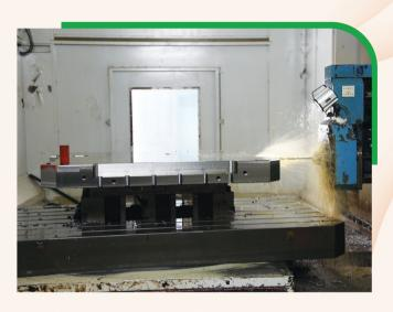
加工中心正為一件大型模架進行加工 A CNC machining centre is processing the machining for a large size mould base
