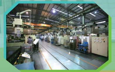
Production line for extra large size mould bases, with over 20 tonnes table loading capacity, to provide services to customers engaged in the manufacturing of auto-parts, and household electrical appliances 超大型模架生產線能加工單件重達20公噸的鋼材以滿足從事汽車、家庭電器用品等客戶的需要
