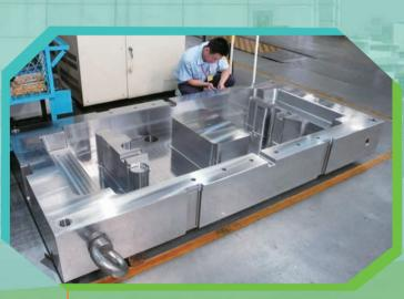
Conducting detailed inspection after subsequent machining processes, to ensure meeting the requirements of customers 大型模架的每一個加工工序後也需要詳細檢測以確保符合客戶的要求
