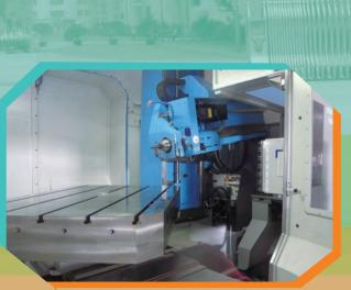
The newly installed 5-axis deep hole-drilling machine is able to produce deep holes on different planes and angles, providing more options in the design of the cooling channels and parts ejecting system
