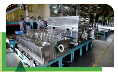
Following the booming of the China big domestic market, the demand for large-sized electrical products and automobile is greatly increased. Lung Kee Group's large-sized mould base production line is well-equipped with advanced precision machineries, capable of providing the quick and comprehensive sub-contracting service for various designs of large-sized moulds.
