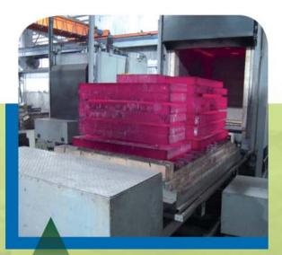
Residual internal stress can result in the deformation of mould plates after cutting and machining processes of steel material. Lung Kee Group's high precision mould bases overcome the problem through careful selection of raw materials together with stress-releasing heat treatment of steel material before machining.
