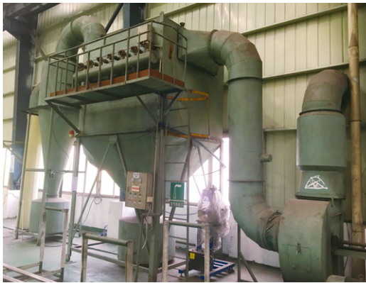
Production plants are equipped with dust collectors with pulse jet filter bags
