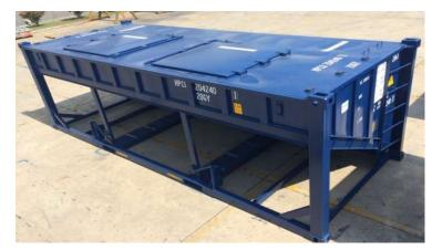
*Mini-box* – 3x12' are bundled by homemade connector for intermodal transportation
