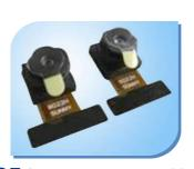
EDOF (extended depth of field) le handset camera module
