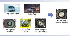
Higher requirements on active resistance to environmental interference: defogging, heating, defrosting and self-cleaning.
