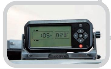
♦ KMB has been progressively installing the tyre pressure monitoring system in its bus fleet, allowing bus captains to monitor tyre pressure and temperature in real time, thereby enhancing bus safety
