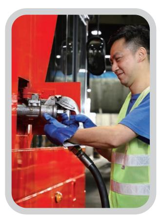
KMB adopts the aircraft-style "Posilock" refuelling system to prevent fuel spillage
