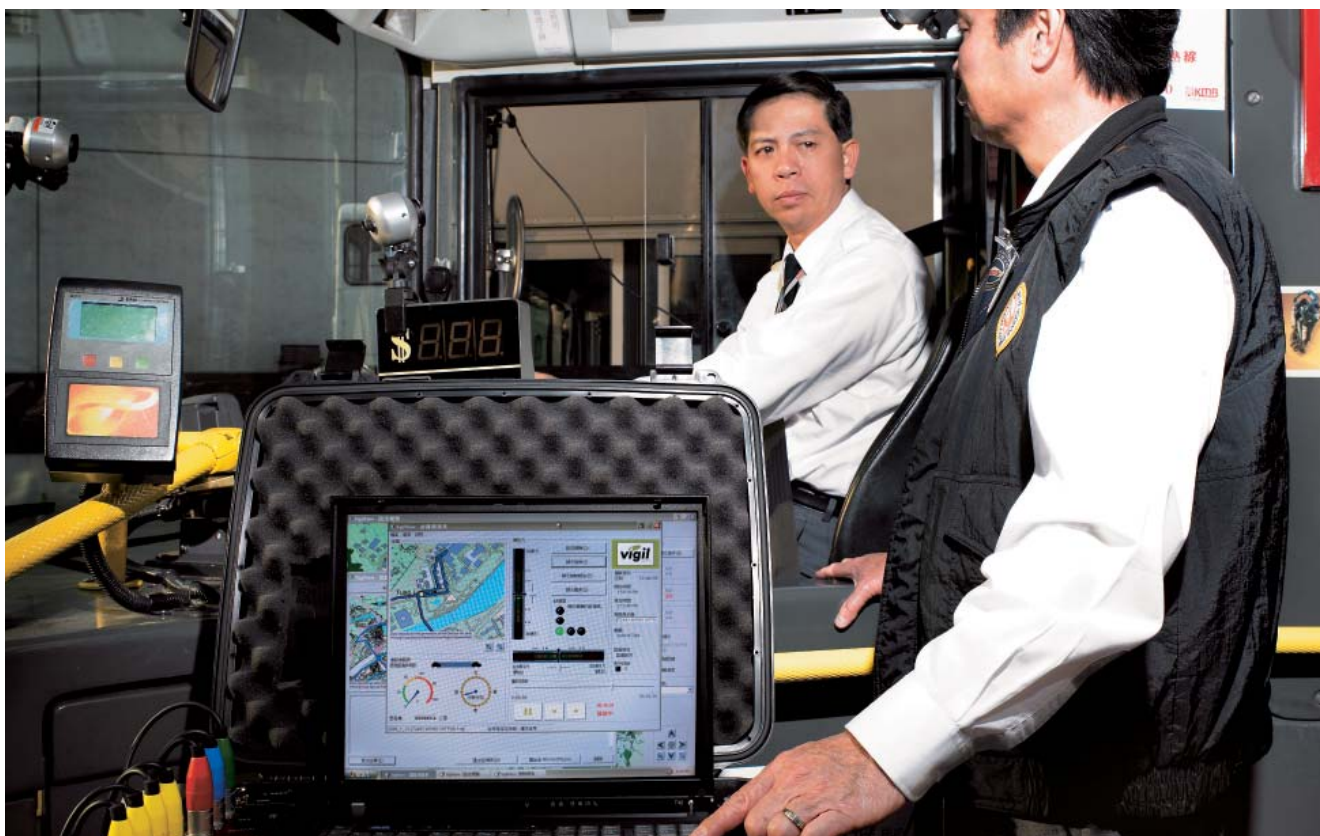
The Vigil Vanguard System is used to assess the driving performance of bus captains in a systematic manner
