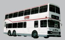
The world's first air-conditioned double-deck bus, developed by KMB, retired from KMB's bus fleet after 17 years of service. The development of this historic bus introduced a new era of double-deckers, using just one engine to control both the driveline and the air-conditioning system. The fuel savings achieved, as well as the environment-friendly design, set new benchmarks.
