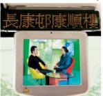
In 1998, KMB and LWB first launched the Electronic Bus Stop Announcement System which delivers voice announcements and shows the name of the upcoming bus stop on LED display on board the bus. All buses are now equipped with such systems.
