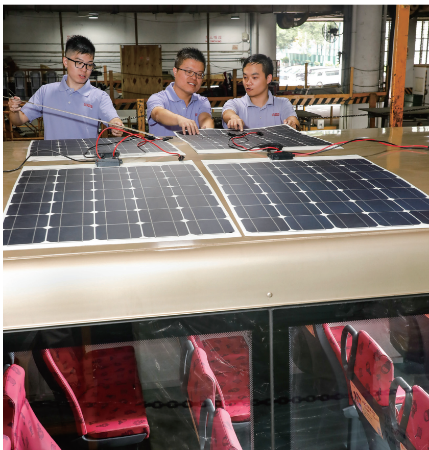
KMB's professional engineering team introduced the first in-house double-deck bus with a solar power system
