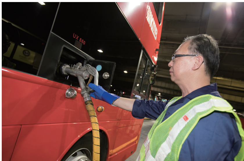
The aircraft-style "Posilock" fuel filling system is used on both KMB and LWB buses to prevent spillage
