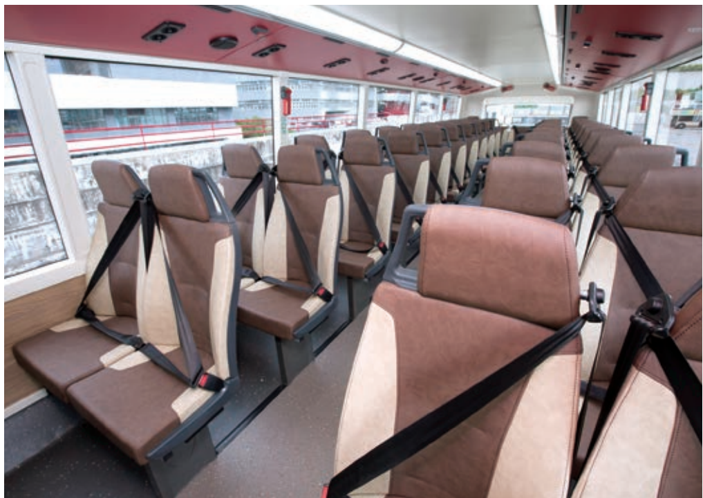
3-point safety belts on all seats have become a standard measure for new buses
