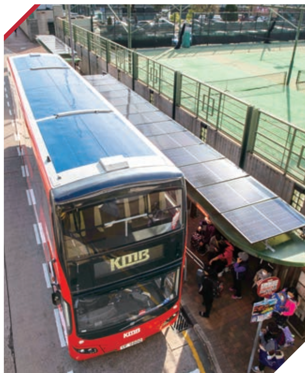
▲ Solar panels installed on the roof of buses have become a standard configuration for newly purchased buses
