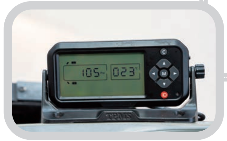
ⓐ KMB has been progressively installing the tyre pressure monitoring system in its bus fleet, allowing bus captains to monitor tyre pressure and temperature in real time, thereby enhancing bus safety
