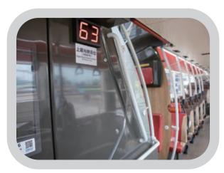
Passengers can notice the number of remaining seats on the upper deck via the device installed on the lower deck
